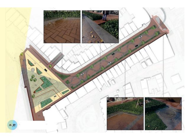
In the pilot project, the street is redesigned as a river that curves to the left so that the water reaches the scouring basin, a former water basin. © Vlissingen
