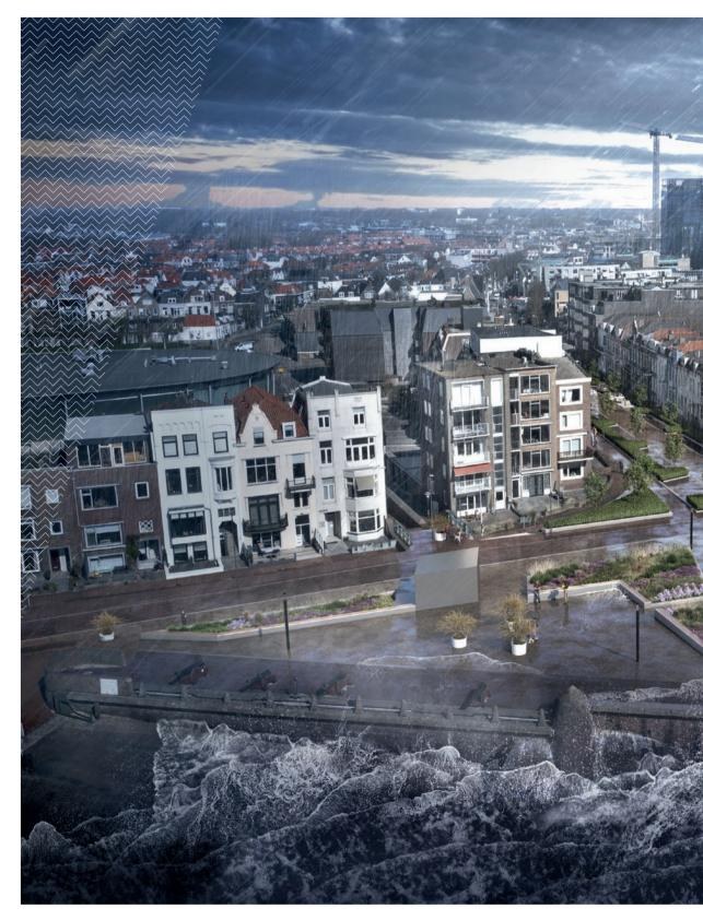
In the incidental situation of a 10,000year storm surge, we let the water flow over the dyke in a controlled way, diverting it to a lower water storage area.
