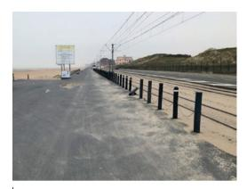
**Existing situation.** At this spot in Ostend, the Koninklijke Baan with its tram tracks runs right along the beach, so the wind blows the sand onto the road and tram rails. Car and tram traffic regularly have to be diverted or interrupted because the sand prevents the flow of traffic.
