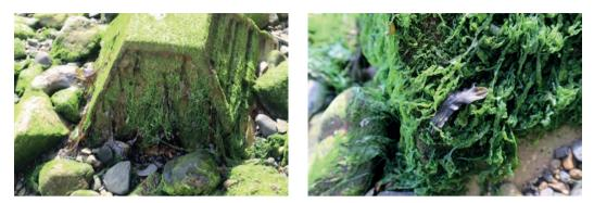
A photo taken in July 2021 of a test eco-block by Exo-Environmental on the test location in Newlyn after the block had been on site for nine months. The dominant sort in the eco-block is *Enteromorpha sp.* (tube algae). *Fucus spiralis* (spiral wrack) is also present.
