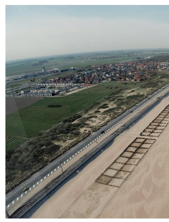
We decided to build a 'dune-before-dyke' over a length of 700 m. The principle is very simple: thanks to the covering of marram grass, the dune will retain the sand, preventing it from blowing inland.
